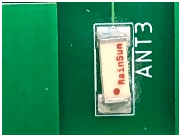
Figure 22 - Rainsun Antenna AN2051-245 on PCB
